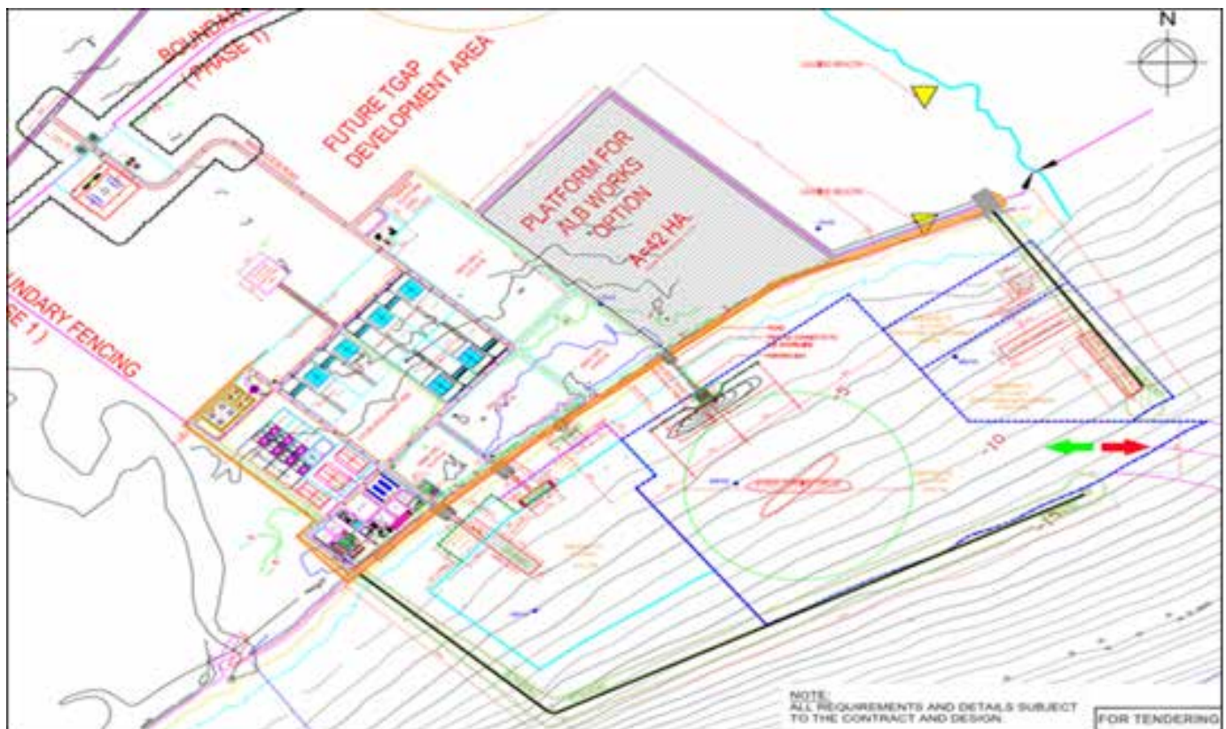
SSB revised master plan, with the additional liquid jetty and required dredging to -14m ACD
