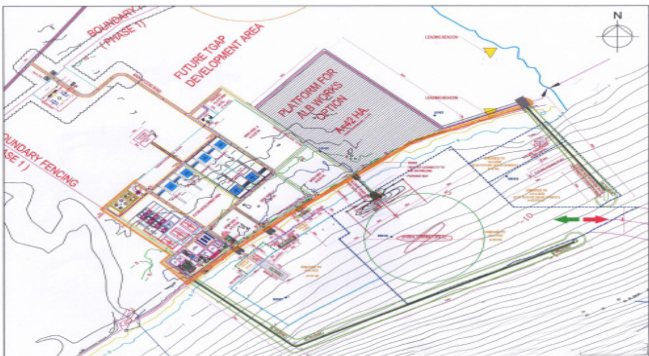
SSB revised master plan, with the additional liquid jetty and required dredging to -14m ACD
