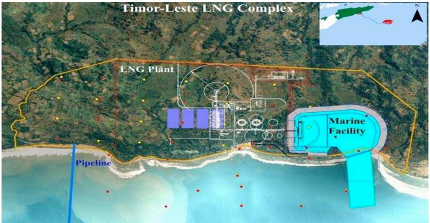
Figure 4-15: LNG Plant, Marine Facility and Pipeline Landing Point (Onshore Section)
