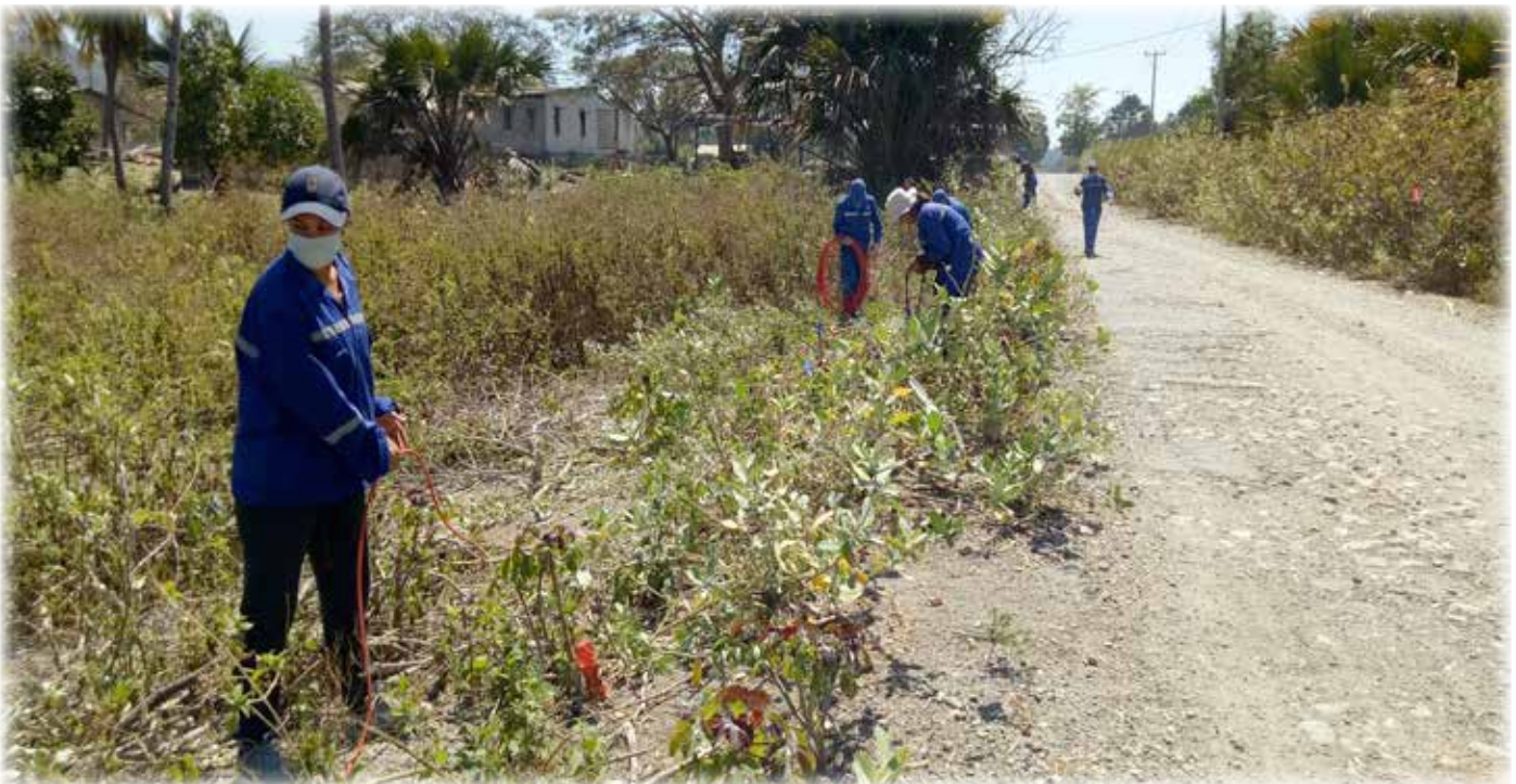
Figure 3-4: TGSS team during planting Geophon
