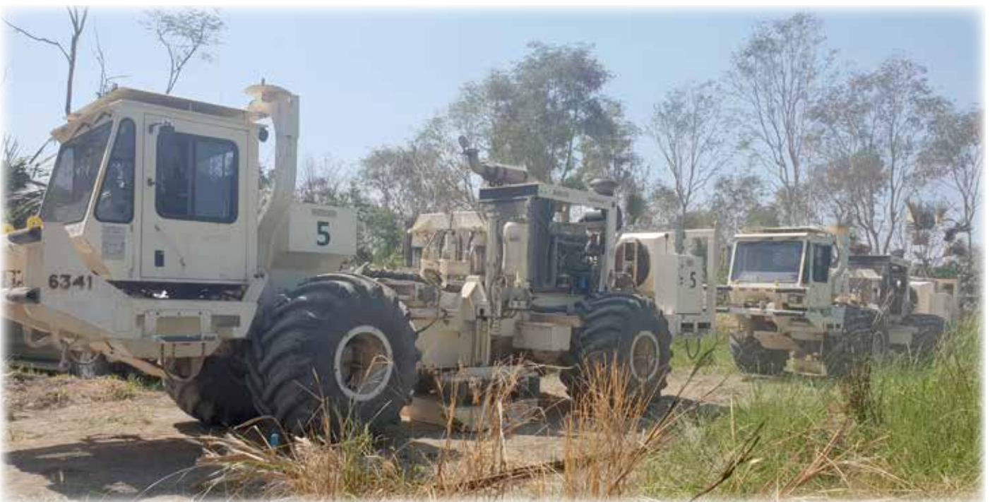
Figure 2-6: Vibroseis trucks during the 2D seismic acquisition in Block C
