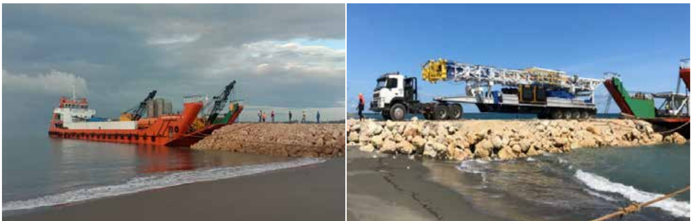
Figure 2-14: LCT Maritindo Perkasa 2 berths at the TR rock causeway port at the Suai (left); Rig Mast unloading (right)
