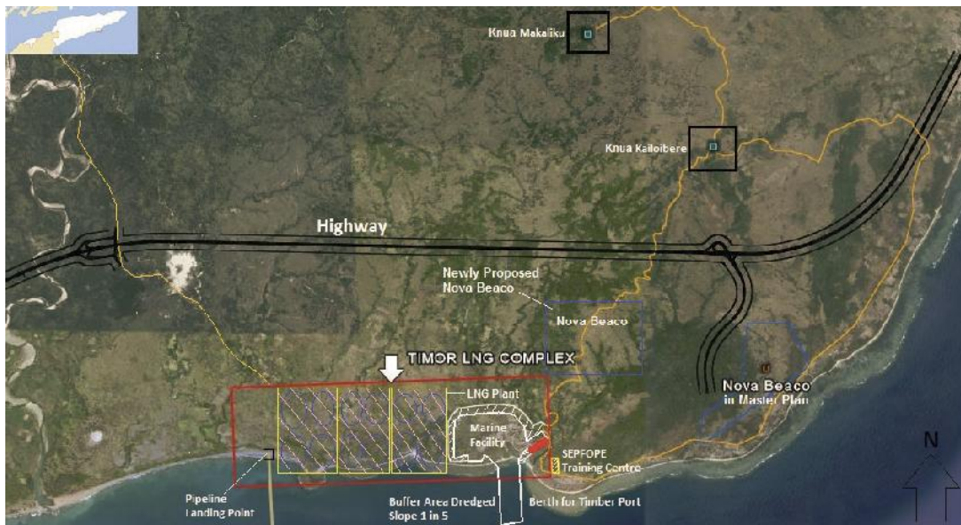
Layout of the Timor LNG Complex, Beaço industrial cluster
