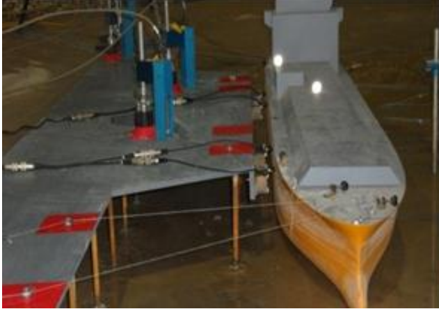
Marine facility physical modelling for FEED testing the strengths of berthing and mooring lines
