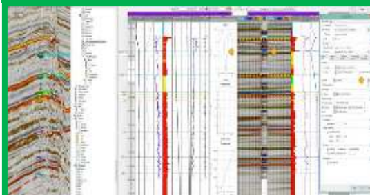
Fig.4: Seismic well tie analysis to synchronize seismic with well
